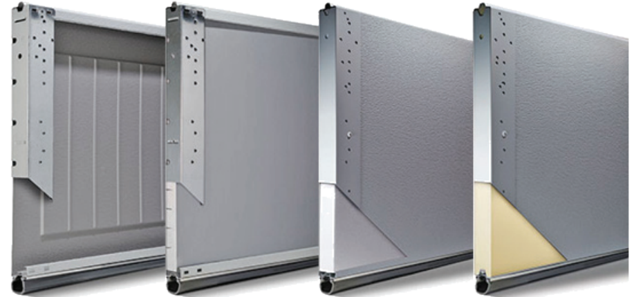
HOLLOW R0 VINYL BACK R7.65 POLYSTYRENE R9.65 POLYURETHANE R17.19
